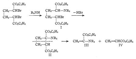
The first step in the reaction is assumed to be the normal replacement of one of the bromine atoms by a dialkylamino group. The cyclobutane intermediate (II) is then produced by the elimination of a molecule of hydrobromic acid. This aminocyclobutane derivative, being unstable under the conditions of the experiment, undergoes dissociation into ethyl acrylate (IV) and ethyl  $\alpha$ -dialkylamino-acrylate (III).
